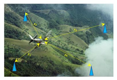
Let there be a right-handed coordinate system fixed to a point on earth. There are N (N = 1, 2, ...) antennas of *known* positions, represented as  $[x_i, y_i, z_i, ]^T$ , i = 1, 2, ..., N, in this coordinate system. A sensor on the vehicle can measure the range to each antenna, giving  $r_i$ , i = 1, 2, ..., N.
